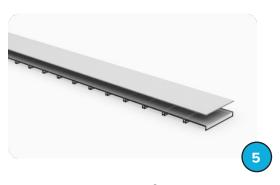
**4.** Then the foam layer (I) can be placed on top of the sections. The dark grey foam should be at the bottom (Fig. 5).
