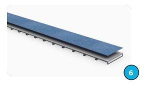
**5.** The blue Triflex Rollmat (E) can then be rolled out (Fig.6).
